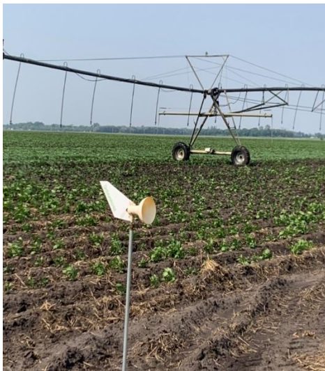
Fig. 12. Passive Spornado spore trap set up at the edge of a potato field. Photo: Vikram Bisht (Manitoba Agriculture).
