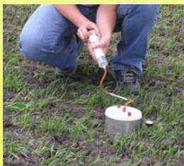
Figure 2. An aluminum ring is driven into the ground and sealed. After ½ hour, the air in this enclosed chamber is drawn through a Draeger detection tube with a syringe.
