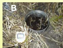
Figure 5. An aluminum ring is driven into the soil. Saran wrap is placed over the soil surface and 1" of water ponded on top. The saran wrap is pulled away to allow the water to start infiltrating (A), which is timed with the stopwatch (B). Measurements are done at least 2 times.
