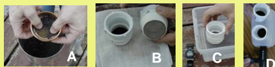
Figure 6. Dry soil is pressed through a screen to sort to aggregate size (A). The soil aggregates are placed on a fine mesh, moistened by resting on a wet cloth (B), and shaken for 3 minutes in water (C). The aggregates that do not "melt" through the fine screen are considered "stable". The sample is dried (D) and weighed to determine the % of the aggregates that are stable.
