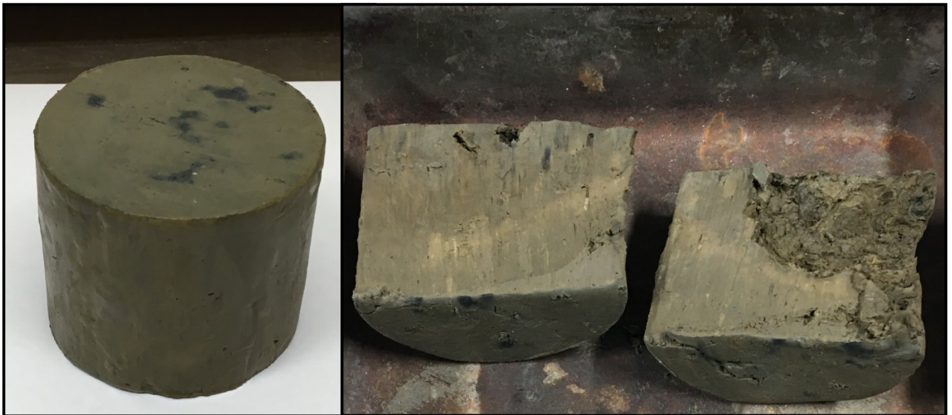
PHOTOGRAPH #2: Sample S7 after completion of hydraulic conductivity testing.
