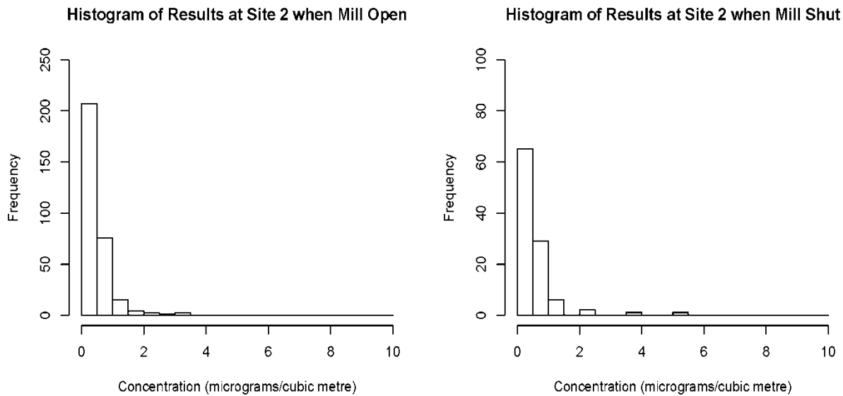
Figure 9: Frequency of samples from Site 2 falling in the indicated 0.5 µg/m 3 width concentration categories for days when the mill is operating (left) and shut down (right)
