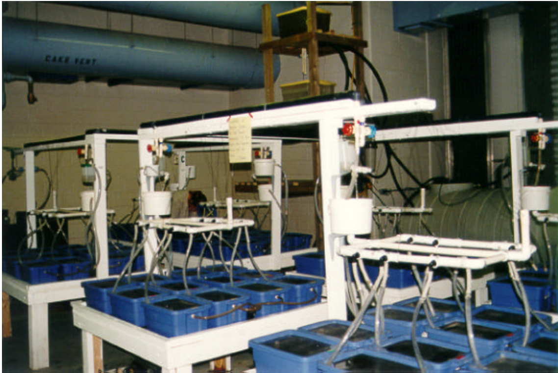
Continuous flow toxicity laboratory within the Dewatering Building at NEWPCC Figure 3-8
