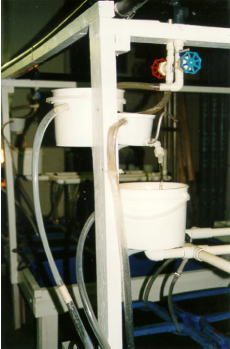
River water and ammonia swing arm diluters at the 0.5mg/L exposure table
