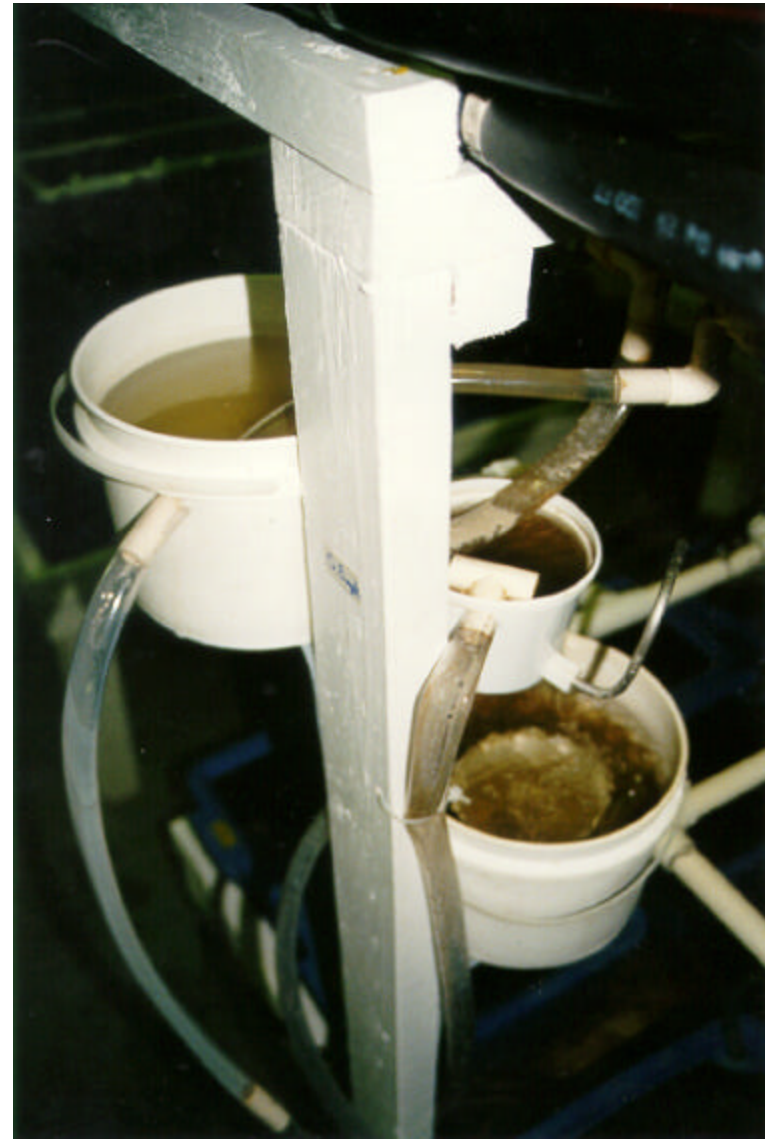
Top view of the river water and ammonia swing arm diluters
