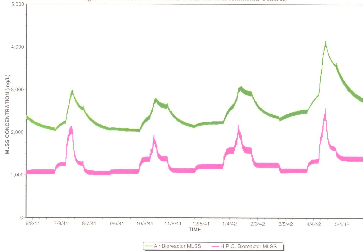
Figure 8.11: Bioreactor MLSS (Modest Level of Ammonia Control)
