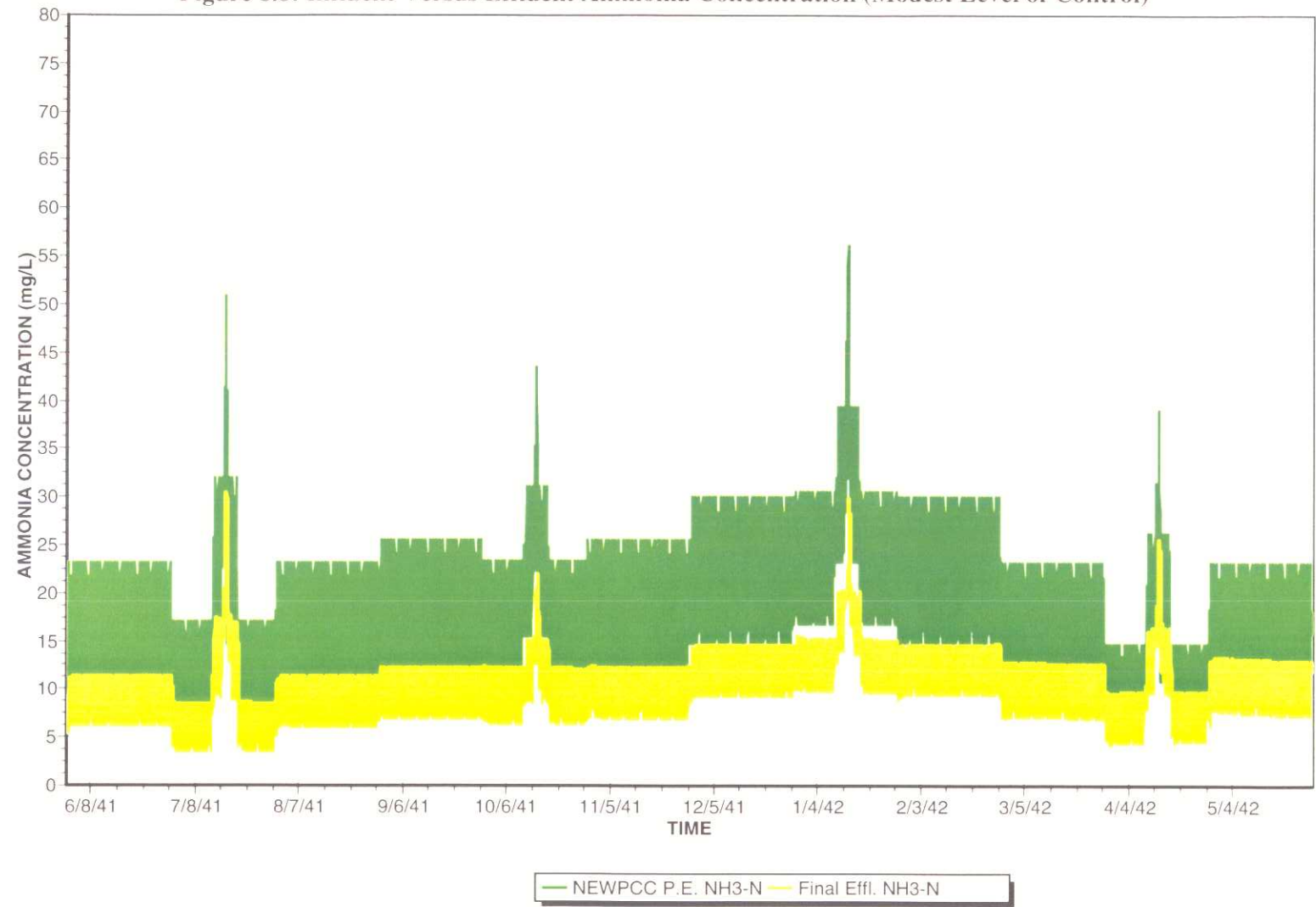
Figure 8.8: Influent Versus Effluent Ammonia Concentration (Modest Level of Control)
