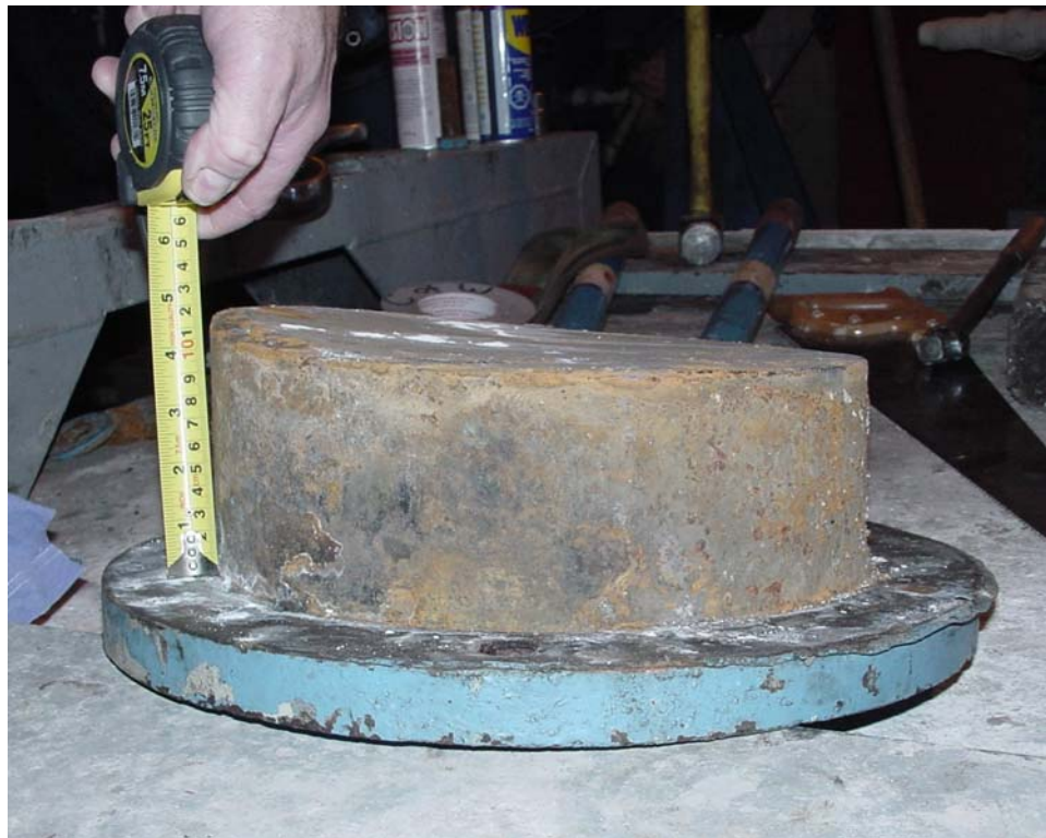
Fig. 3.1 - Views of the Inspection Plate after the event. The plate weights about 90 pounds.
