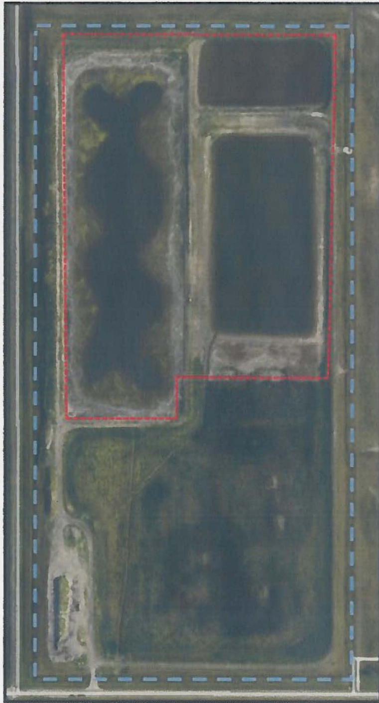
Figure 5. Proposed 1.2 m fencing location around perimeter of old lagoon site (light-blue, dashed line) and proposed 1.8 m fencing on the inside of the lagoon berms around areas remaining under licence (i.e., control, holding, and wetland cells). Note that the fencing locations shown are approximate and for discussion purposes only. Image courtesy of Google Earth (Imagery date: 2013).
