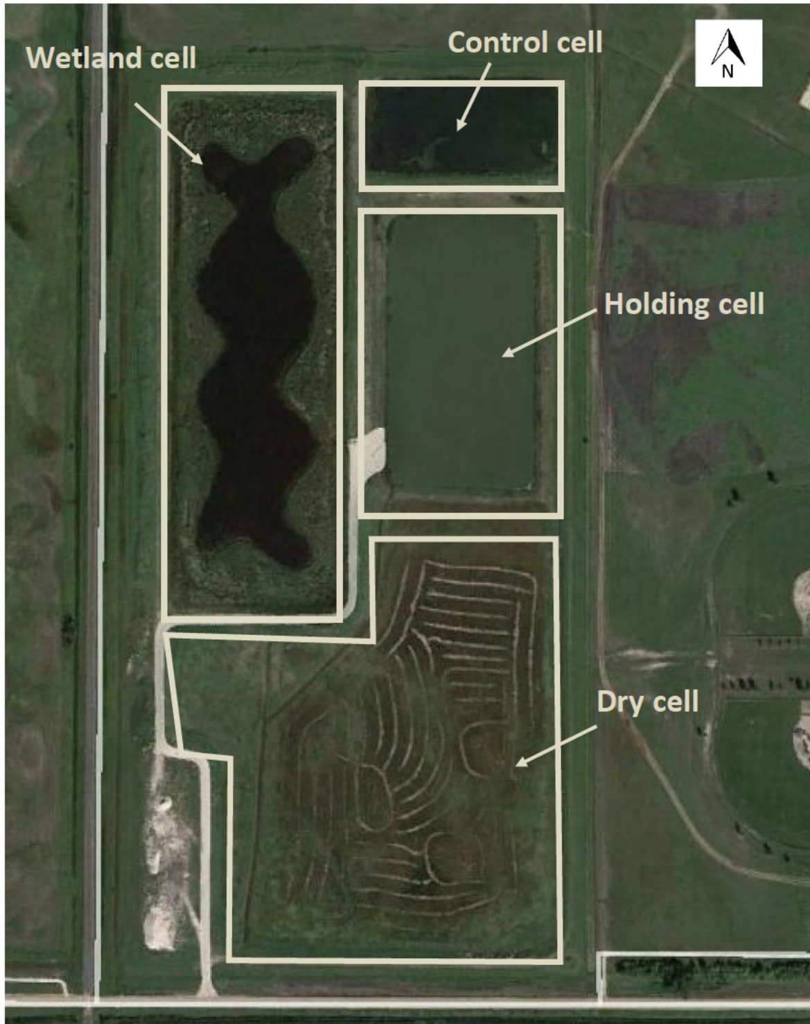
Figure 1. Niverville lagoon phytoremediation project site, including the wetland cell, control cell, holding cell and dry cell. Image courtesy of Google Earth (Imagery date: 2016).
