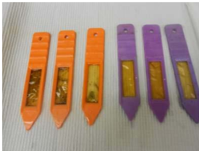
Figure 5. PRS probes retrieved from a research plot in the Niverville wetland cell, cleaned and combined to form a composite site for the plot.
