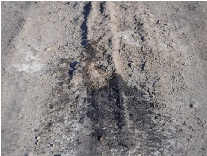
Photo 2: PHC (oil) staining clay soil
