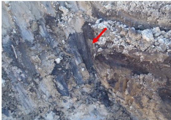
Photo 1: Grey-black PHC, PAH, and/or PCB soil staining
