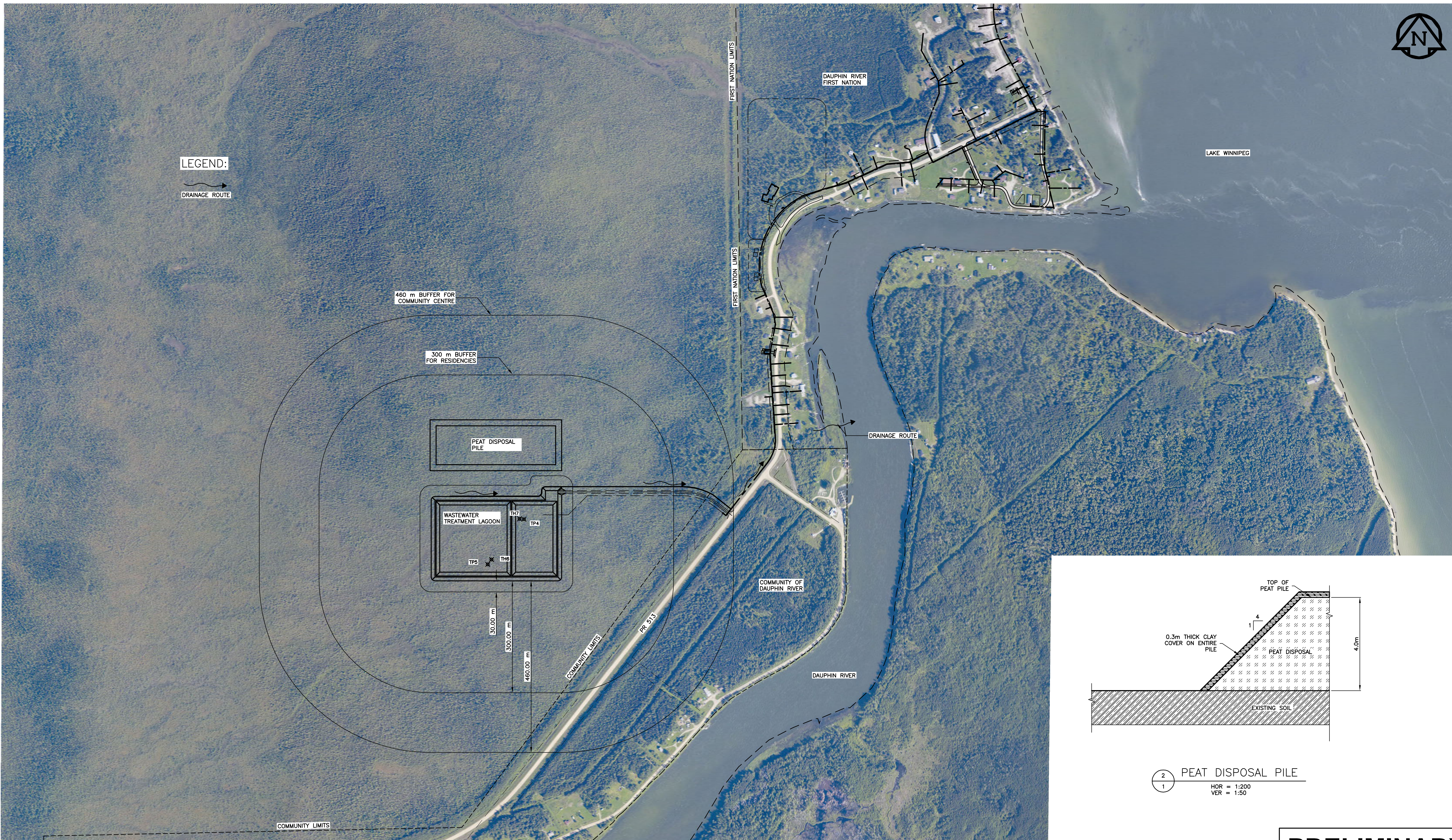
1 PROPOSED LAGOON WITH TEST HOLE LOCATION, DRAINAGE ROUTE AND SETBACK PLAN SCALE = 1:5000
