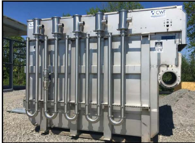
Figure 1: GEM System (To be housed within the shipping container building). Source: Veolia Water Technologies
