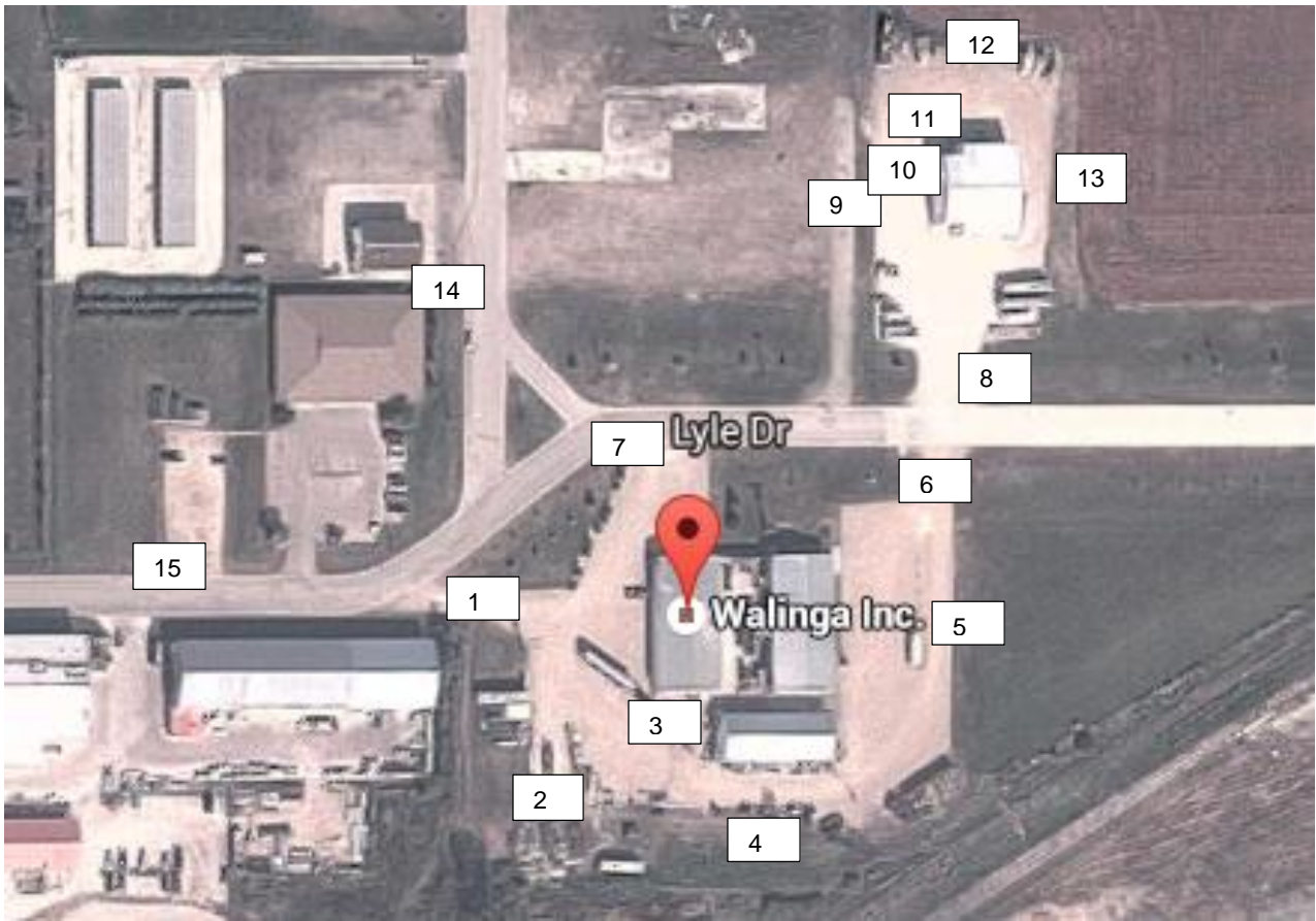
Overhead of View Showing Locations of Noise Testing
