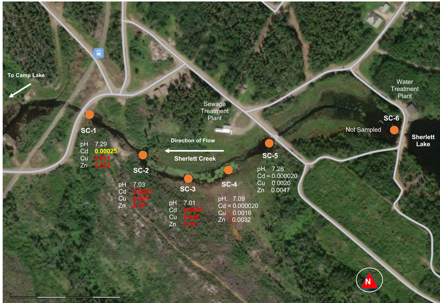
Figure 21. Sherlett Creek detailed sampling locations with pH (field), total cadmium (Cd), total copper (Cu), and total zinc (Zn) concentrations on 26 July 2021. Values in white are within MWQSOG Tier II objectives; values in yellow exceed the Tier II chronic exposure objectives; and, values in red exceed the Tier II acute exposure objectives.
