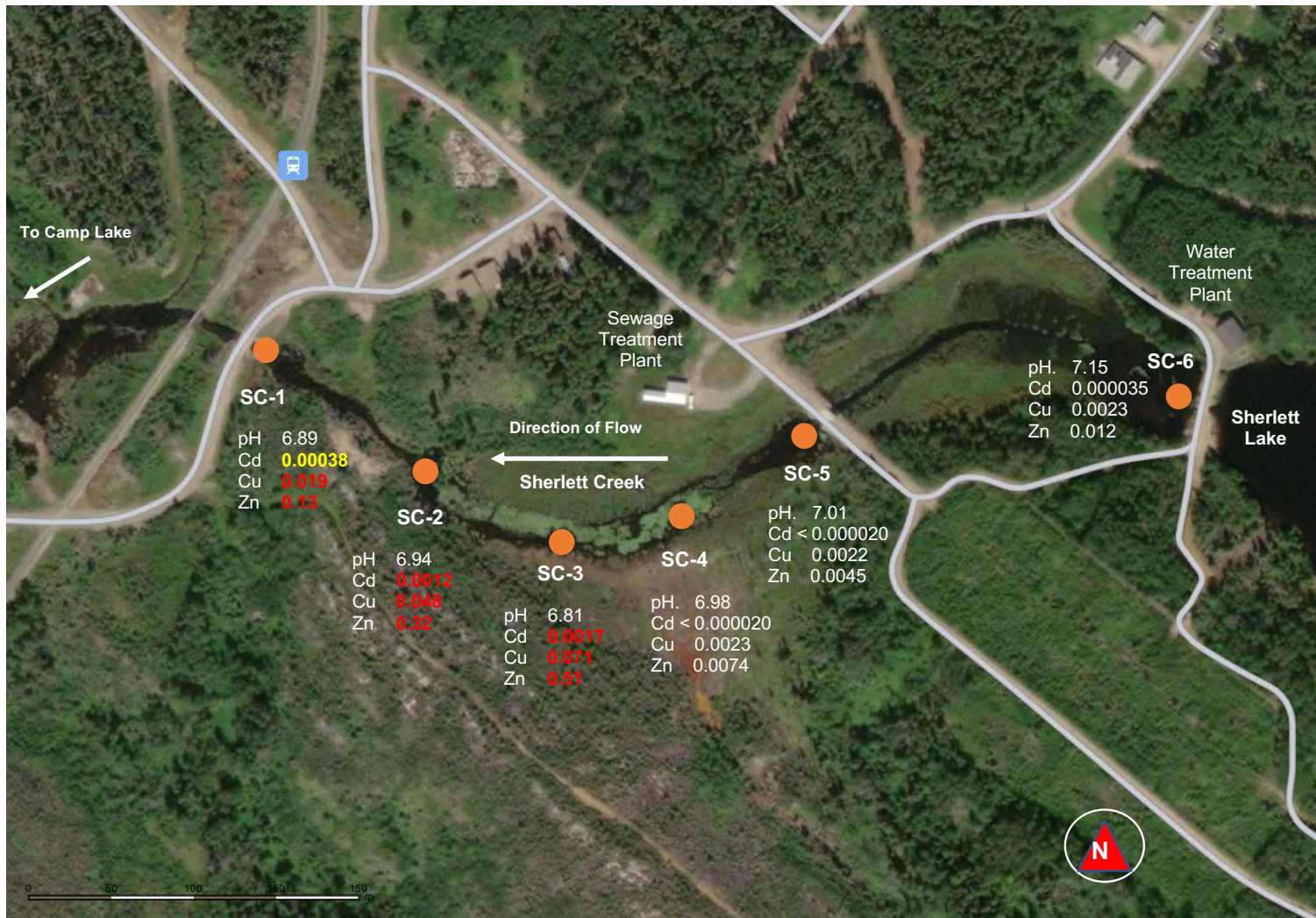
Figure 20. Sherlett Creek detailed sampling locations with pH (field), total cadmium (Cd), total copper (Cu), and total zinc (Zn) concentrations on 18 July 2021. Values in white are within MWQSOG Tier II objectives; values in yellow exceed the Tier II chronic exposure objectives; and, values in red exceed the Tier II acute exposure objectives.
