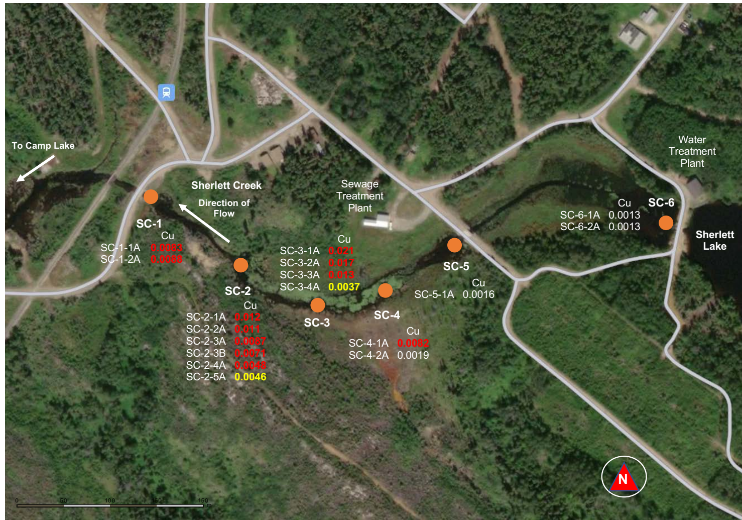
Figure 24. Sherlett Creek detailed cross-section samples, 22 August 2021 – total copper (mg/L). Samples with an “A” designation were collected from near surface. Samples with a “B” designation were collected from near bottom. Values in white are within MWQSOG criteria; values in yellow exceed the Tier II chronic exposure objective; and values in red exceed the Tier II acute exposure objective.
