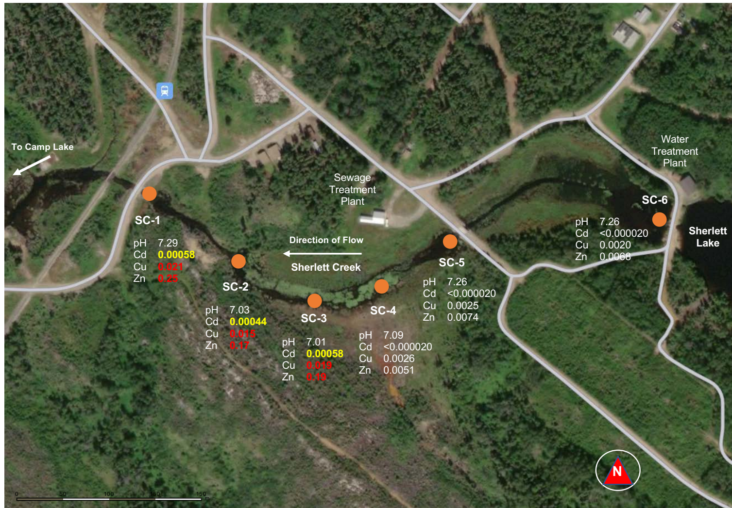
Figure 26. Sherlett Creek detailed sampling locations with pH (field), total cadmium (Cd), total copper (Cu), and total zinc (Zn) concentrations on 5 Sep 2021. Values in white are within MWQSOG Tier II objectives; values in yellow exceed the Tier II chronic exposure objectives; and, values in red exceed the Tier II acute exposure objectives.
