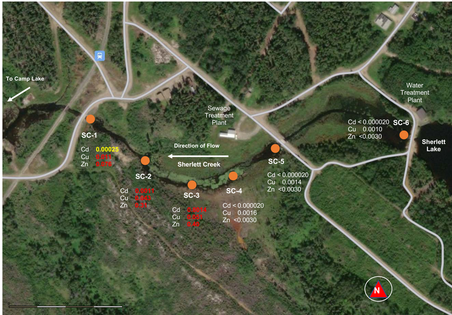
Figure 22. Sherlett Creek detailed sampling locations with total cadmium (Cd), total copper (Cu), and total zinc (Zn) concentrations on 9 August 2021. Values in white are within MWQSOG Tier II objectives; values in yellow exceed the Tier II chronic exposure objective; and, values in red exceed the Tier II acute exposure objective.
