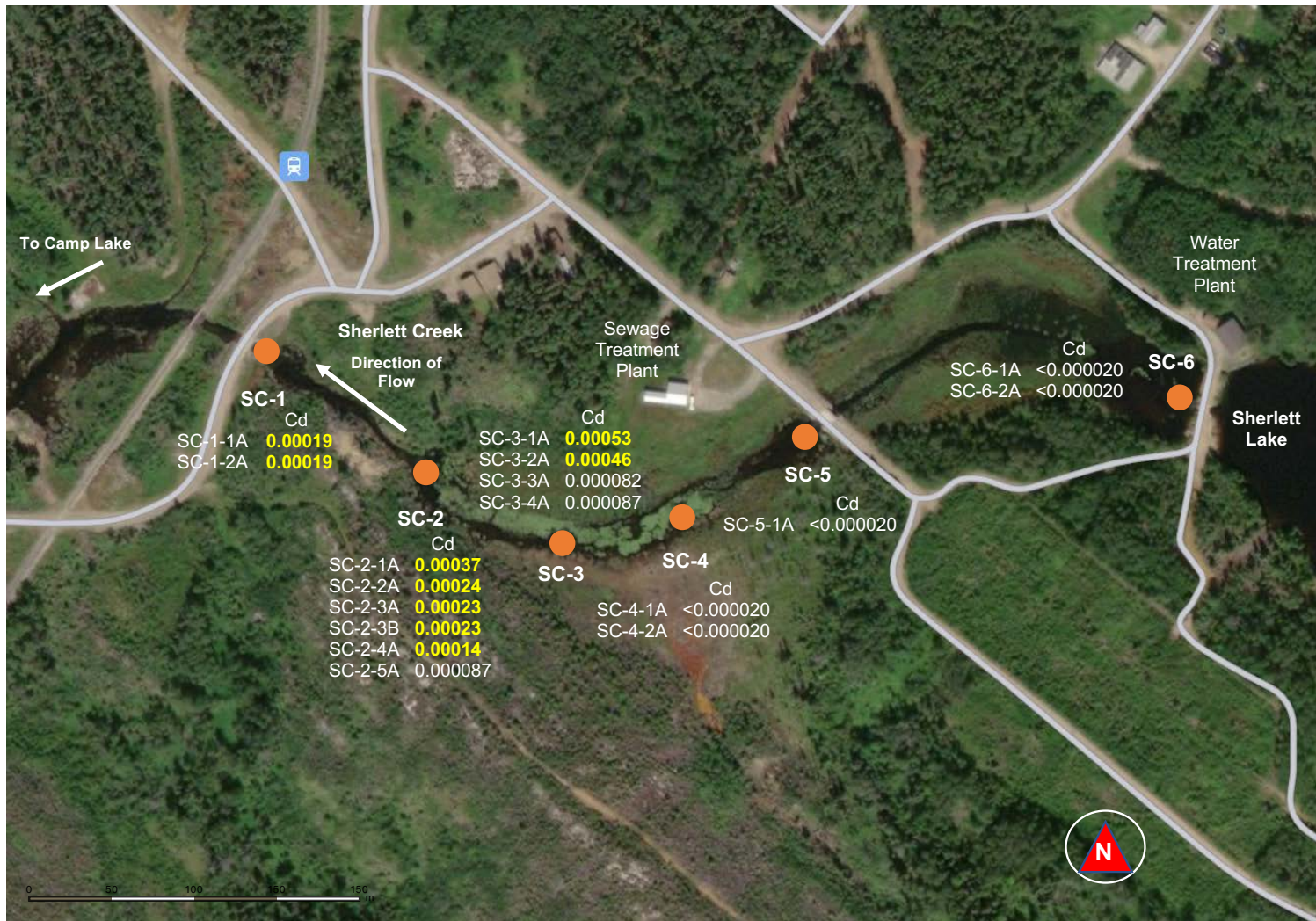
Figure 23. Sherlett Creek detailed cross-section samples, 22 August 2021 – total cadmium (mg/L). Samples with an “A” designation were collected from near surface. Samples with a “B” designation were collected from near bottom. Values in white are within MWQSOG criteria; values in yellow exceed the Tier II chronic exposure objective; and values in red exceed the Tier II acute exposure objective.
