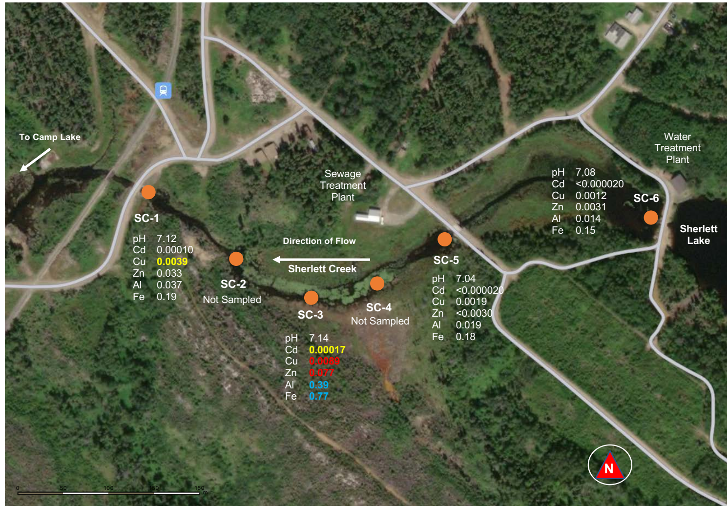
Figure 29. Sherlett Creek detailed sampling locations with pH (lab), total cadmium (Cd), total copper (Cu), total zinc (Zn), total aluminum (Al), and total iron (Fe) concentrations on 1 February 2022. Values in white are within MWQSOG criteria; values in blue exceed the Tier III guidelines; values in yellow exceed the Tier II chronic exposure objectives; and values in red exceed the Tier II acute exposure objectives.
