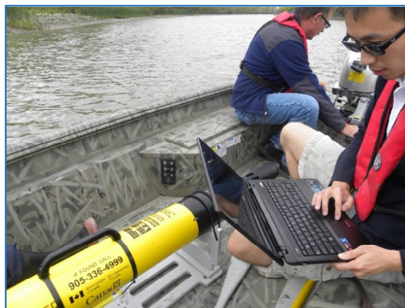
Downloading water quality data from a data sonde.
